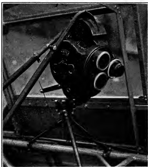
FIG. 1. Set-up of camera for photographing instrument board during dive test.
